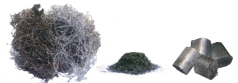
Pressing of the shredded swarf into handy briquettes.
